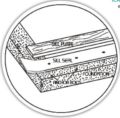
ICA Sill Seal is a ribbed, non-crosslinked polyethylene foam that seals the gap between the foundation and the seal plate.
